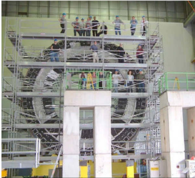
Fig. 5. First Tile Calorimeter cylinder fully pre-assembled on the surface and ready for installation underground (April 2003)
