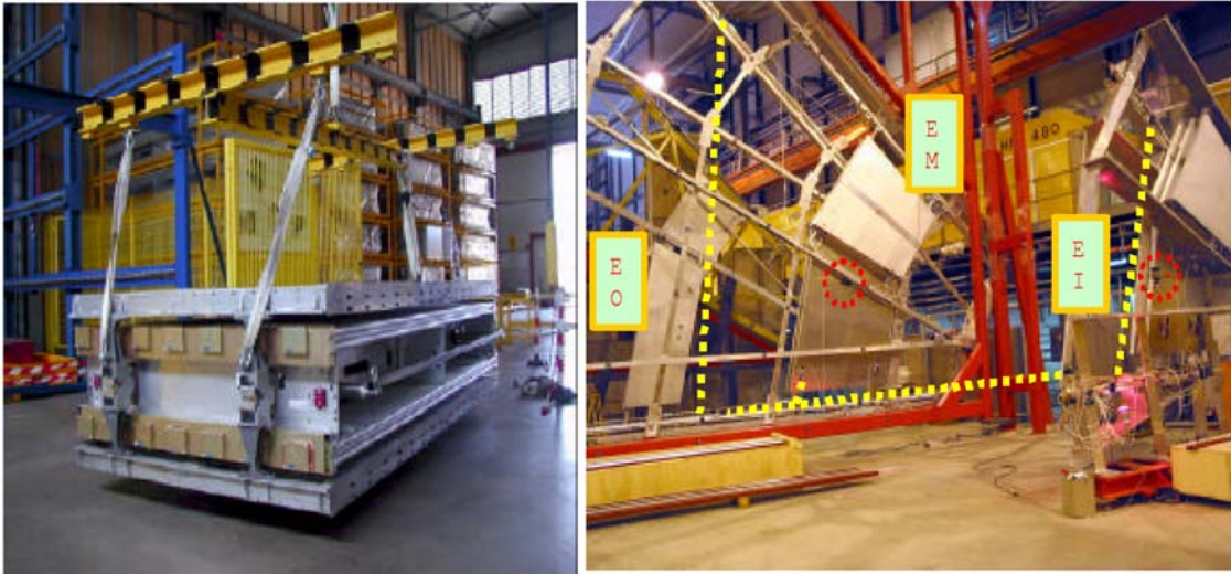
Fig. 7. a First MDT+RPCS assembly. b Test beam test stand in the SPS H8 beam line
